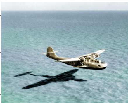
The sea wings, or sponsons, on the Martin M-130 provided improved stability on the water plus the added advantage of each carrying 950 gallons of fuel.
